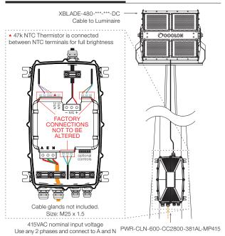
Distance between the power supply and luminaire can be extended up to 100 metres using a min 1.5mm<sup>2</sup>.
