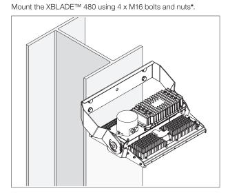
**NOTE:** XBLADE 480 can rotate 360°. Please be aware of the power cable's position with respect to the angle of the luminaire, avoid cable damage due to excessive bending. When using the locking / securing screws 1 screw per side will be sufficient however some angles allow for an additional screw if desired.
