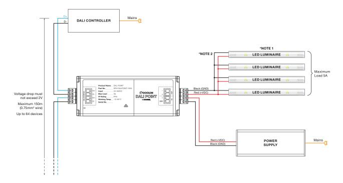
\*NOTE 1 DO NOT EXCEED maximum single of each luminaire check individual product specifications for run length.
