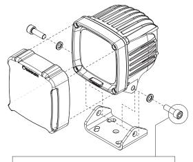
Recommended Torque 37 Nm Max Torque 48 Nm
