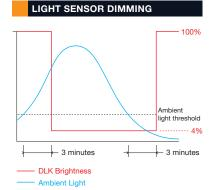
The DLK LED will be at 100% brightness when it is turned on and then will dim to 4% brightness when daylight is detected. 3 minutes after the daylight has dropped below the minimum ambient light threshold, the DLK LED will ramp up to 100% brightness. (Only applies to DLK equipped with light sensor)
