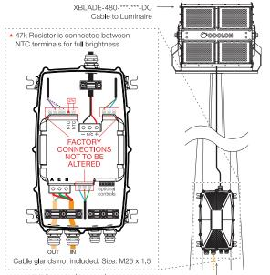
415VAC nominal input voltage Use any 2 phases and connect to A and N  $\,$
